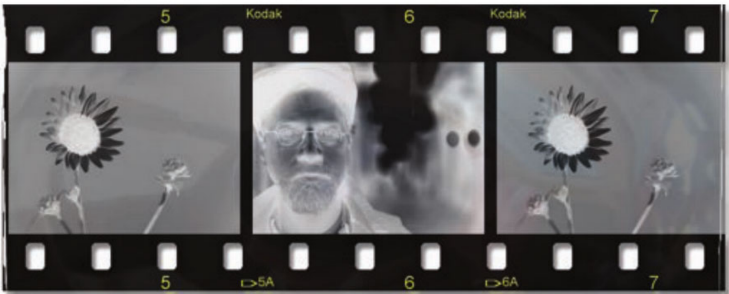
Figure 1.1 After a piece of film is developed, it contains a negative image.
